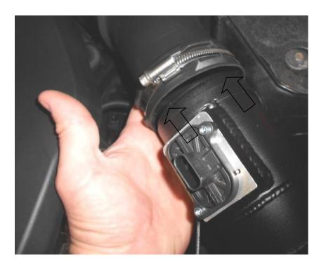
34. Reconnect the wiring to the MAF sensor.
