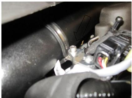
19. Feed the intake pipe into position and plug-in the blowby heater (if fitted to the vehicle) and reconnect the wiring.
