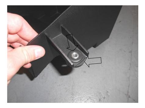
31. Carefully fit the airfilter tray in position and secure with the M6x20mm Allen bolt and 6mm penny washer.
